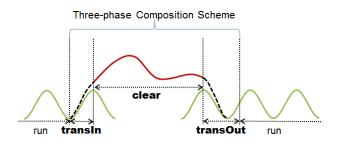
**Figure 5:** *Three-phase composition scheme and control blending. The solid lines are the control quantities for the individual skills, and the dashed lines are the blended quantities for transitions.*
